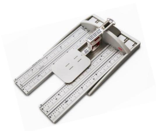
The new ADE MZ10042 portable stadiometer is ideally suitable for field workers as well as for PGs and hospital use. The height rod can be quickly taken apart into 4 pieces which can be stored within the platform. The two wall distance pieces keep the height rod steady and vertical at the wall without any additional fixing. The scale can be read from both sides at the clear red indicator point.
