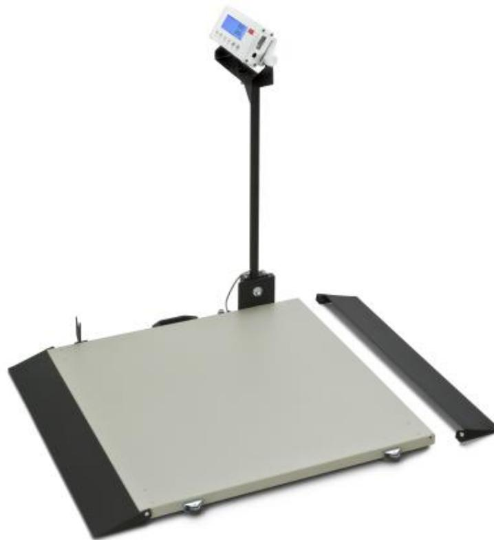
Low level platform scale with one ramp for convenient access. The cable remote LCD display with blue backlit shows the weight clearly and can be mounted to the wall with the supplied support bracket. Two castors and one handle permit a quick transport. Powered by mains and rechargeable batteries, allowing the use of the scale at any place. It is equipped with a practical display holder to allow readings close to eye level. A second ramp can be purchased as optional accessory ref. MZ30010.
