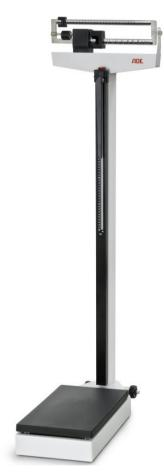
Eye-level beam scale, readable from both sides, equipped with a telescopic height measuring rod as standard and two transport castors for easy movability. This solid and robust scale is made of steel and comes with a heavy-duty cast-iron lever system, guaranteeing a long and trouble-free life time. The large base is covered by a removable none slip cover for easy cleaning and secure use.
