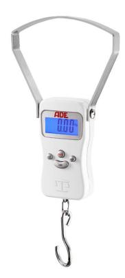
Electronic baby hanging scale - small and practical device made of coated aluminum, with integrated length measuring tape and a fixed hook made of galvanized metal for weighing slings. The large folding handle made of blasted stainless steel provides an extra secure hold and allows newborns to be weighed quickly and safely. The scale weighs babies up to 20 kg with an accuracy of 20 g. The LCD with blue backlight enables clear reading even in low light conditions.
