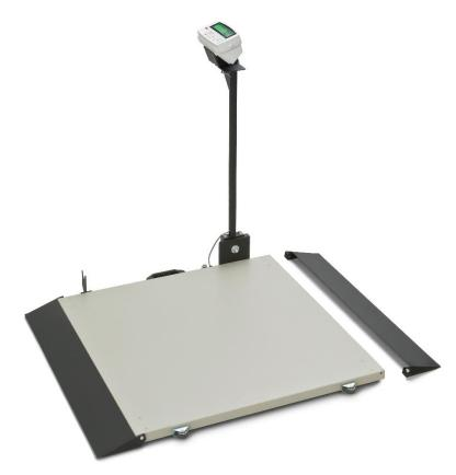
Low level platform scale with one ramp for convenient access with wheel chairs and foldable display holder column. Two castors and one handle permit a quick transport. The pre tare function will allow you to deduct a memorized weight just by pressing one button. Such the net weight of a patient can be determined. A hold and tare function will help to get a quick and precise reading of the patient's weight. Powered by mains and rechargeable batteries.
