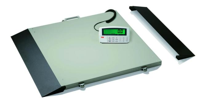
Low level platform scale with one ramp for convenient access with wheel chairs. A cable remote display shows the weight clearly and can be mounted to the wall. Two castors and one handle permit a quick transport. The pre tare function will allow you to deduct a memorized weight just by pressing one button. Such the net weight of a patient can be determined. A hold and tare function will help to get a quick and precise reading of the patient's weight. Powered by mains and rechargeable batteries.
